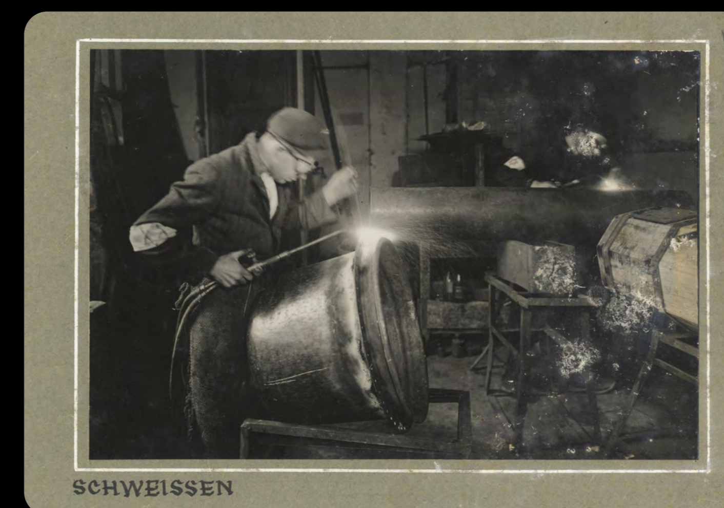
Welding a water boiler in a workshop for manufacturing boilers in the Warsaw ghetto, apparently during 1941.
